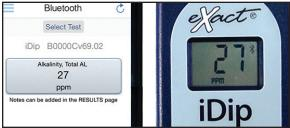
When all tests have been performed, tap 'Results' at the bottom of the screen. To add notes tap the desired test result.
