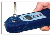
Press (EROID) and the iDip<sup>®</sup> display reads O<sub>PPM</sub> indicating the meter is ready to test. For Standard Liquid Method, place Cell Cover on CELL before zeroing.
