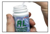
Press **(READ)** to initiate a 20 second countdown and simultaneously **DIP** the test strip by submerging all pads in the sample then use a gentle constant back and forth motion (2 strokes per second) until the timer displays "1". Remove and discard the strip. Wait for count-up time if required.
