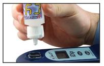
Place the Cell Cover onto the CELL. Press GEAD and a 20 second countdown begins. Turn the meter upside-down repetitively during the 20 seconds. When the timer displays "1", place the iDip® on a flat surface. Wait for count-up time.
